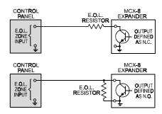
Figure 8. WIRING E.O.L. Zones
